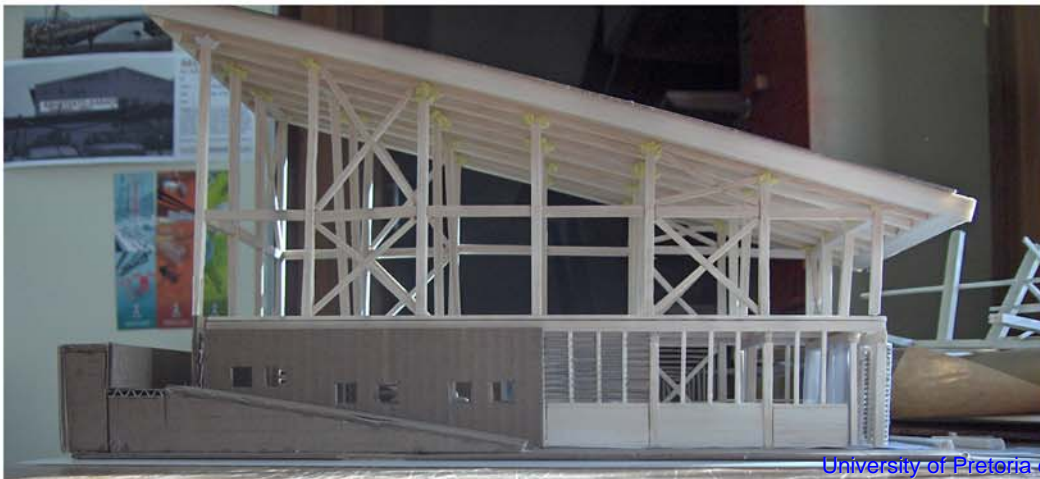
FIG. 165: 1:50 STRUCTURAL WORKING MODEL (AUTHOR, 2006).
