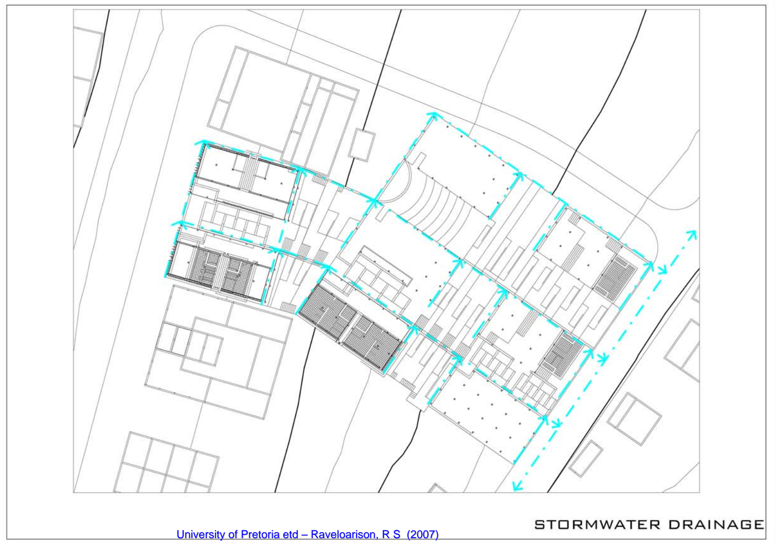
FIG. 168: SITE PLAN WITH STORM WATER DRAINAGE FLOW DIAGRAM (AUTHOR, 2006).
