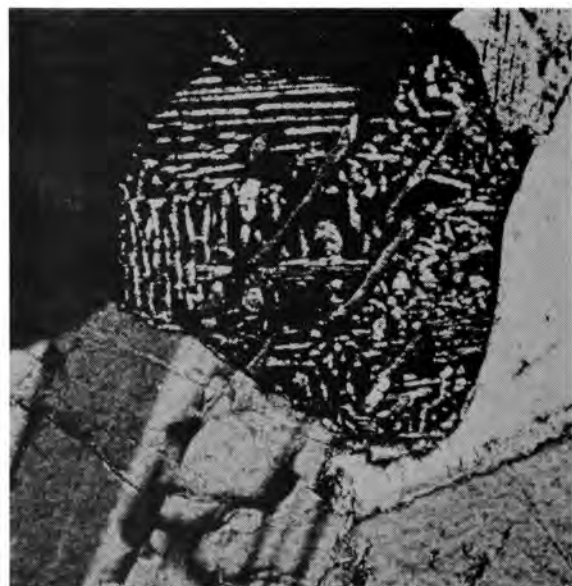
Fig. 39. A grain of inverted pigeonite (in extinction) which contains two sets of post-inversion exsolution-lamellae of augite. Horizontal lamellae parallel to (100), vertical lamellae parallel to (001), diagonal lamellae exsolved prior to inversion. G460, Mapochsgronde 500 JS. Crossed nicols, x75.
