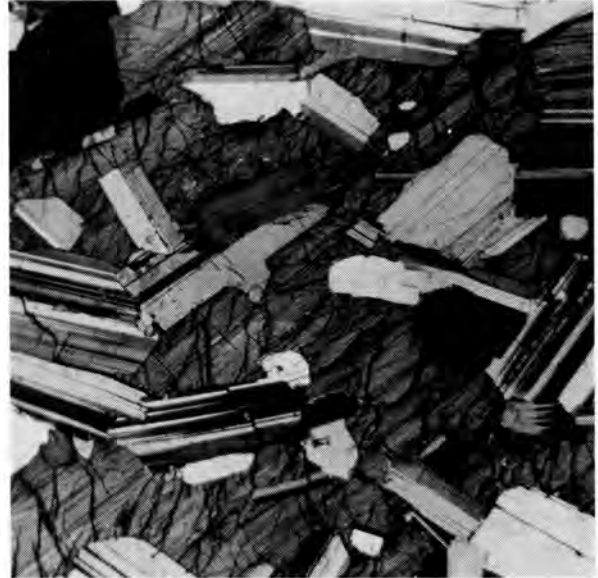
Fig. 34. Primary ophitic orthopyroxene. Specimen PB 717. Crossed nicols, x20.
