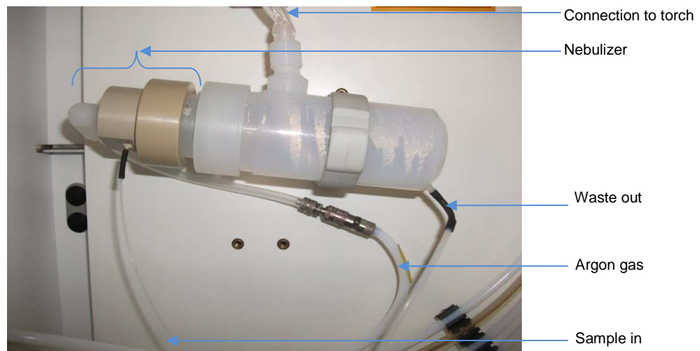
Figure 39. Spray chamber connected to the nebulizer.
