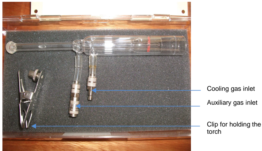
Figure 41. An image of a torch for Spectro Arcos.
