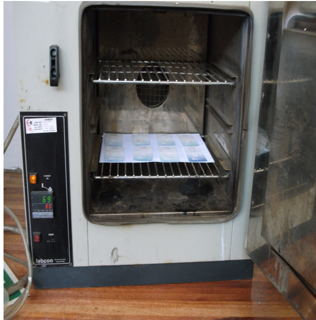
Figure 41: Experimental set up for accelerated temperature ageing
