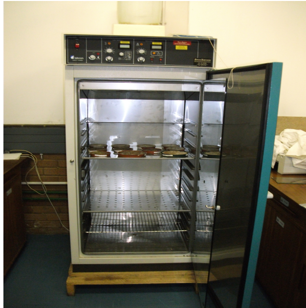
Figure 43: Experimental set up for accelerated humidity ageing
