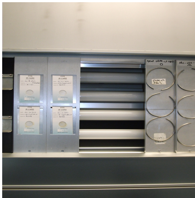
Figure 42: Experimental set up for ultra-violet light ageing: note the infra red card is facing away from the UV lamps.
