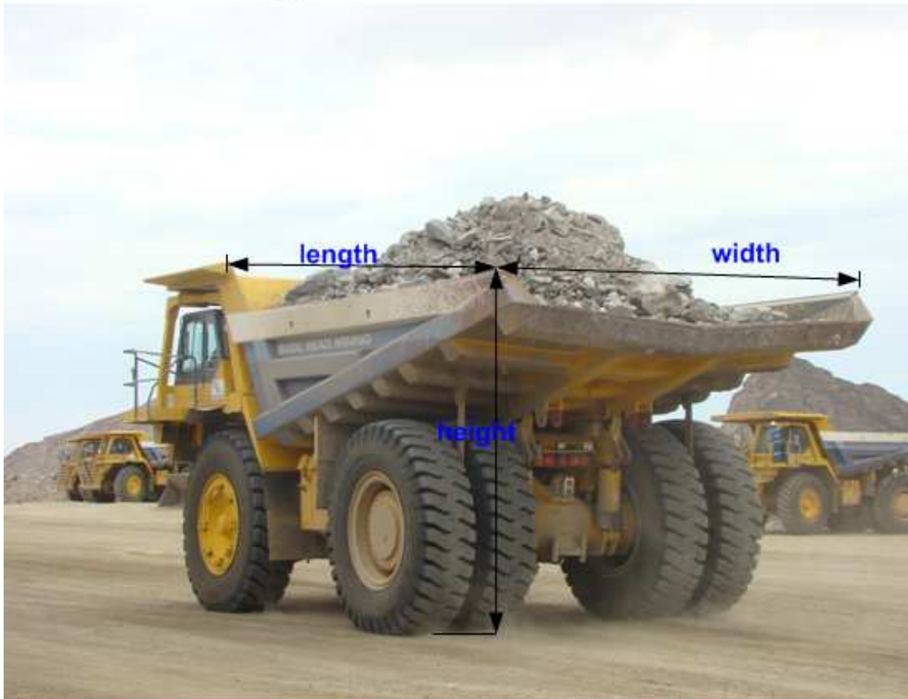
Figure 3.4: The dimensions of the haul truck
