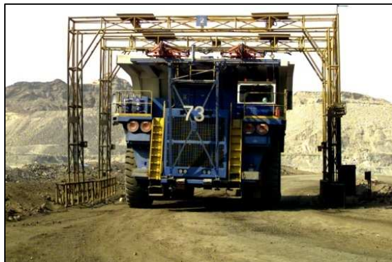
Figure 2.5.: Radiometric scanning of the ore loaded on the haul truck
