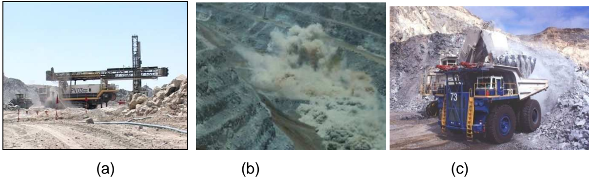
Figure 2.4: Different stages of mining operations at Rössing Mine (a) drilling in progress (b) blasting (c) loading of ore into a truck by means of hydraulic shovel (Pictures courtesy of RUL)
