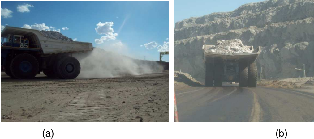
Figure 3.8 Unpaved roads (a) with no Dust-a-Side (b) treated with Dust-a-Side
