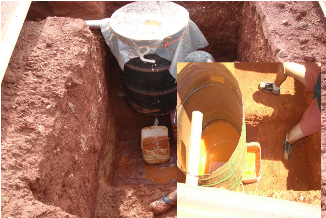
FIG. 4.2: Runoff measurement using collection tanks and small containers Hatfield Experimental Farm
