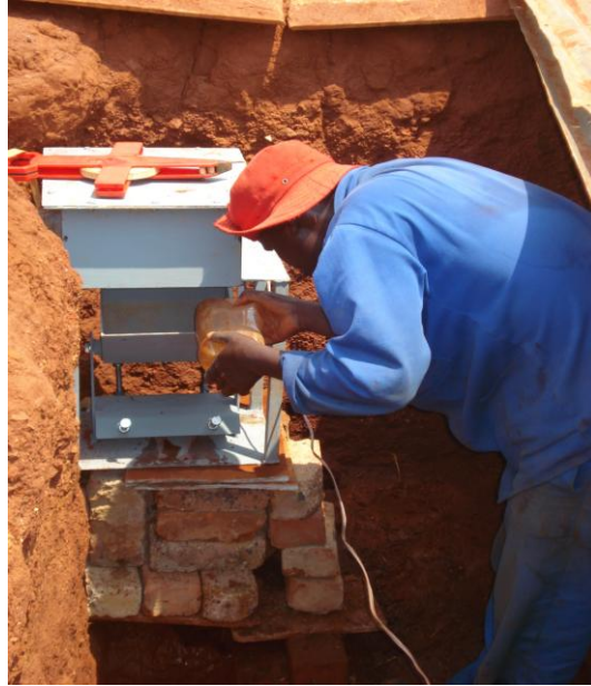
FIG. 4.4: Calibration of a tipping bucket runoff meter under field conditions, Hatfield Experimental Farm
