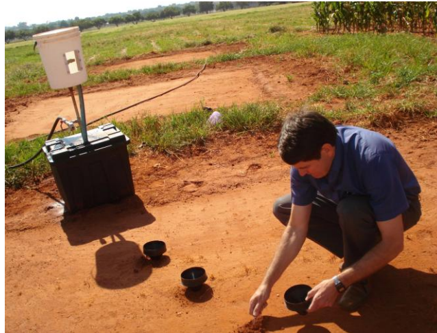
FIG. 4.7: Sprinkler infiltrometer set up for soil infiltration measurements, Hatfield Experimental Farm
