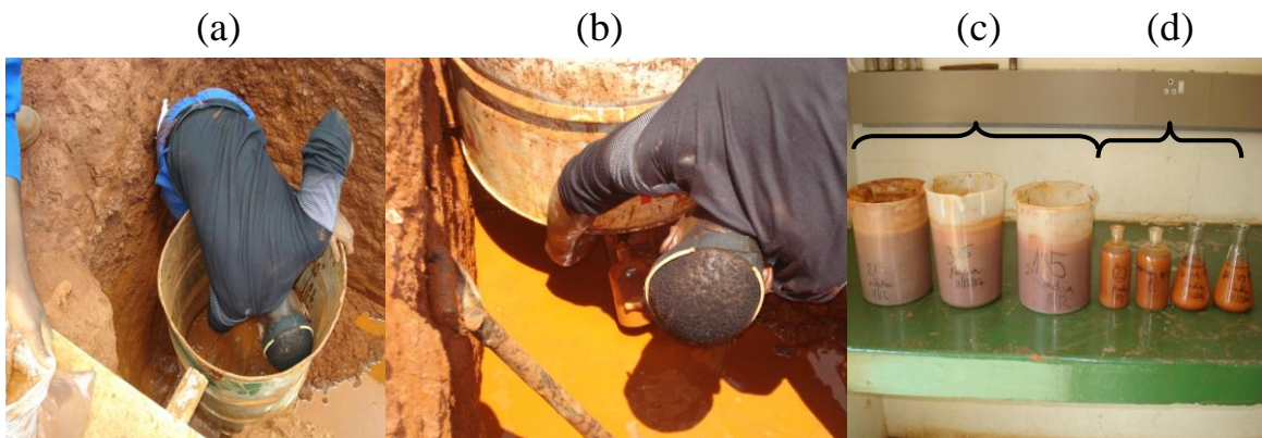
FIG. 4.5: Soil collection from the bottom of the drum (a), from the valve (b), 5 ℓ containers with soil from the bottom of the drum from different earthen runoff plots (c), and 500 ml containers with soil samples from the valve (d), Hatfield Experimental Farm
