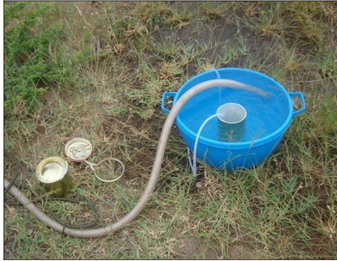
Photo 1. Photograph of discharge hose, canisters and glass bottles used for the CFC sampling.
