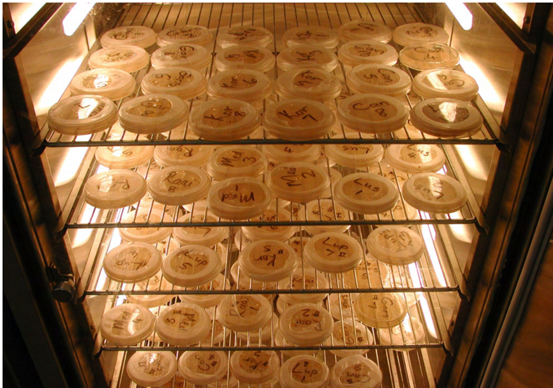
Figure A3 Petri dishes with seeds to obtain leachates in the incubator
