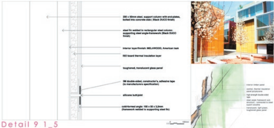
detail 9 layered cladding panel, translucent glass, ISO-board, thermal-insulation, MELAWOOD timber panel
