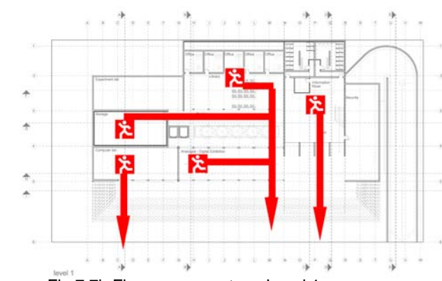
Fig 7.7b Fire escape routes - Level 1
