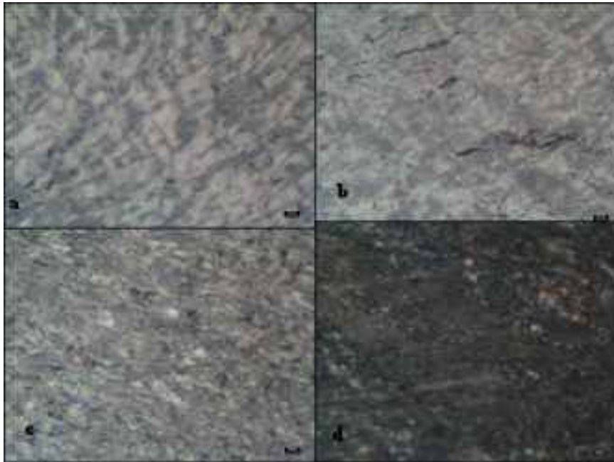
Figure 7.3.16: Optic micrographs of the graphitised cokes showing poor graphitised surface as the dosage of acetylene black is increased
