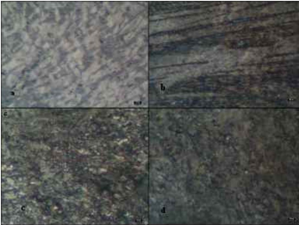
Figure 7.3.17: Optical micrographs of the graphitised cokes showing poorly graphitised surface as the dosage of carbon black is increased
