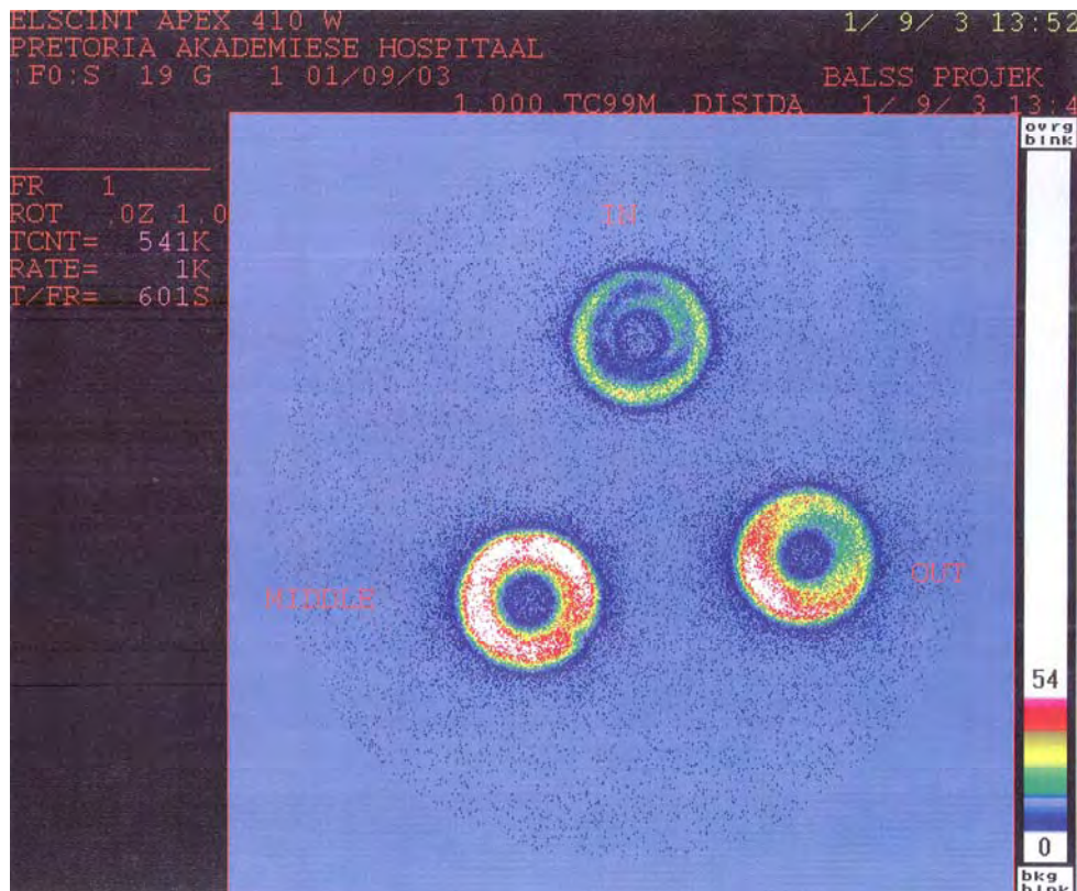
Figure 4.2.4 ^{99m}\text{Tc} -DISIDA isotope scan of PUF cell aggregation matrix. The radial-flow foam was sectioned into inlet, middle and outlet portions along the axis of the
