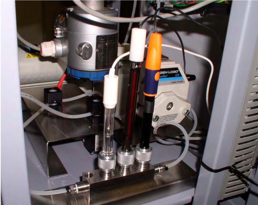
Figure 6.3.2 UP-CSIR BALSS FI sampling manifold with ion-specific electrodes. From left to right carbonate ( \text{HCO}_3^- ), potassium ( \text{K}^+ ) and ammonium ( \text{NH}_4^+ ) electrodes, with peristaltic pump and controller in the rear.
