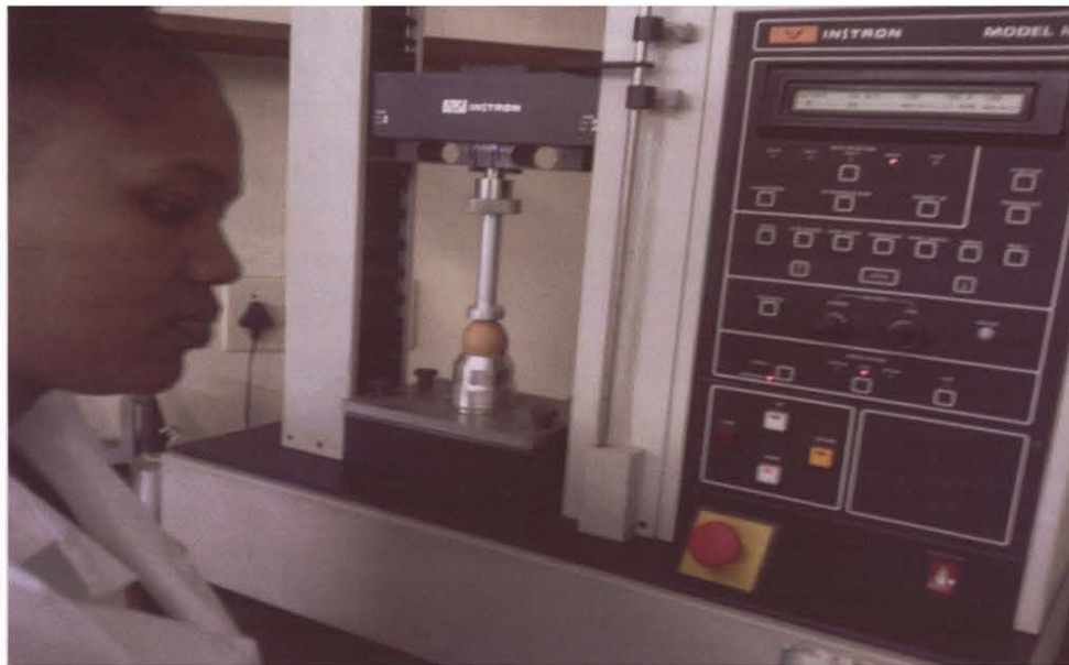
Figure 3.9 Measuring egg shell strength using Instron 10111
