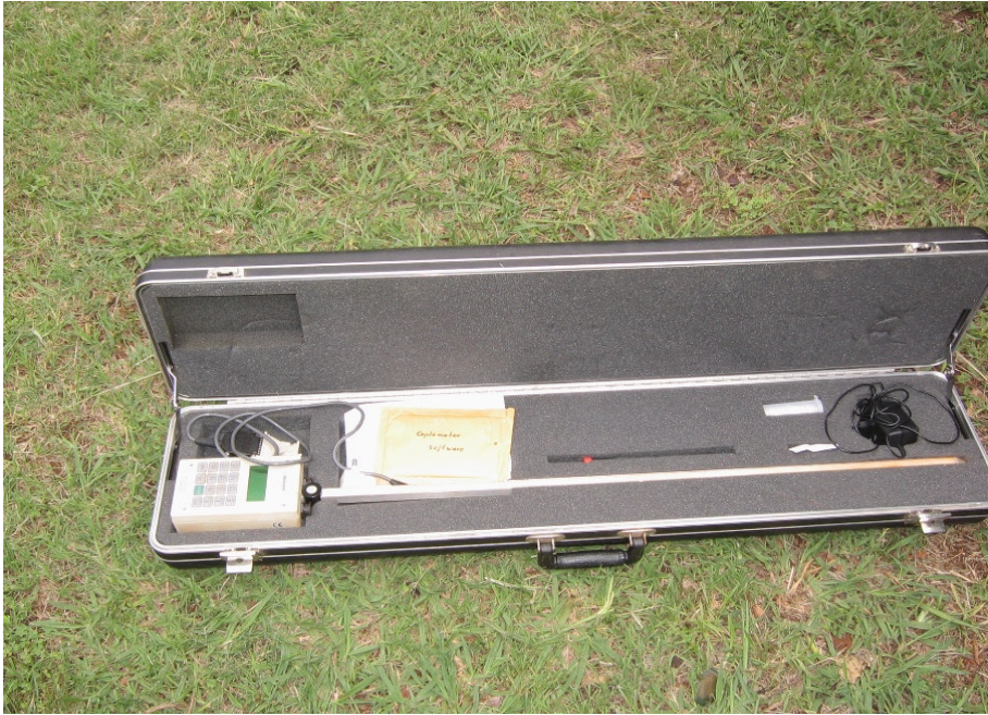
Figure A3 The sunflecks ceptometer, model AccuPAR, used to measure PAR.
