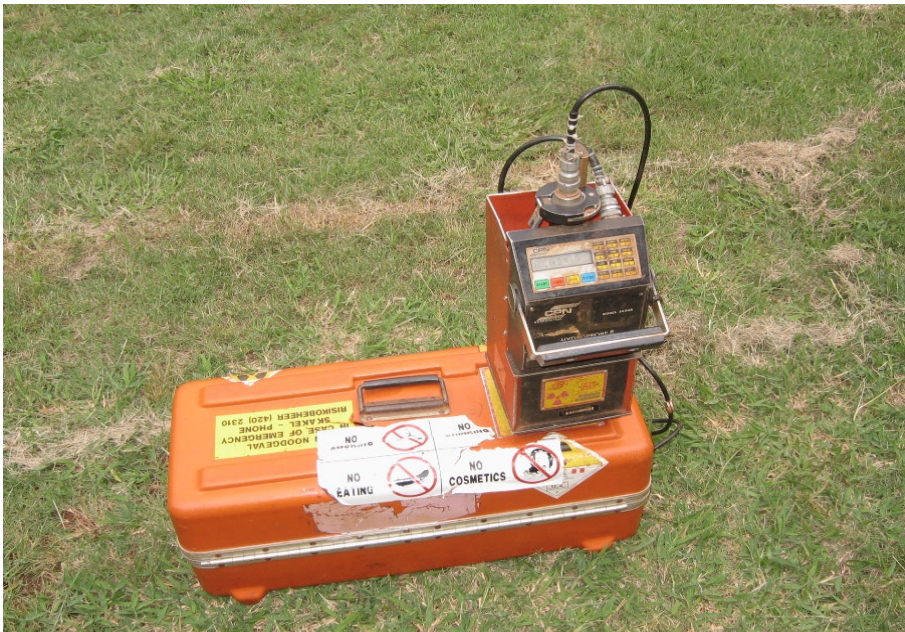
Figure A2 The Hydro probe neutron water meter, model 503DR CPN, used in the Experiments.
