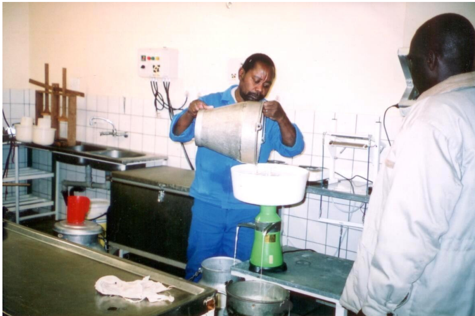
Figure5.3: Cream separation for butter and ghee making
