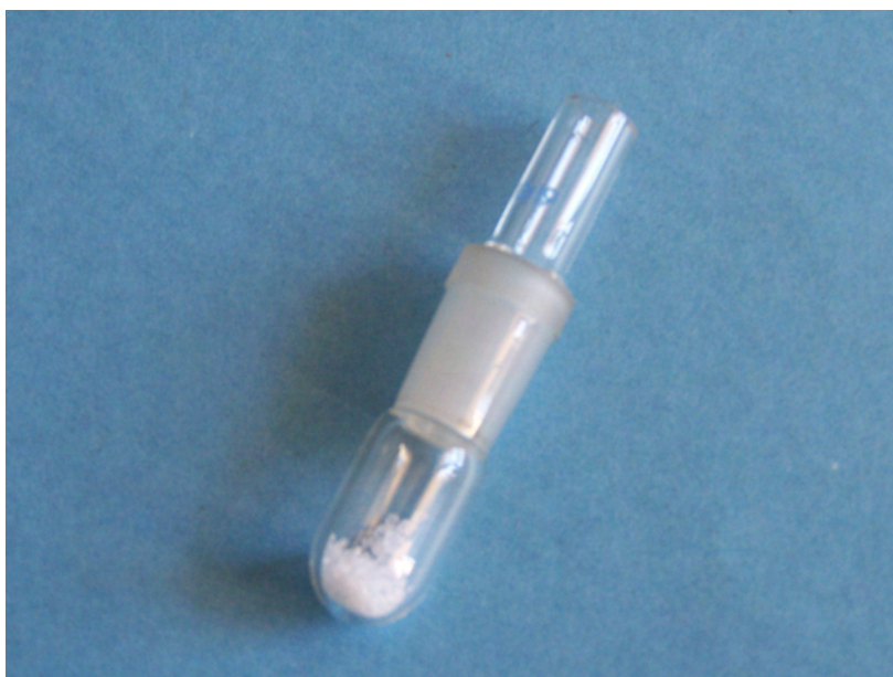
Figure 2.7: Naphthalene diffusion tube.
