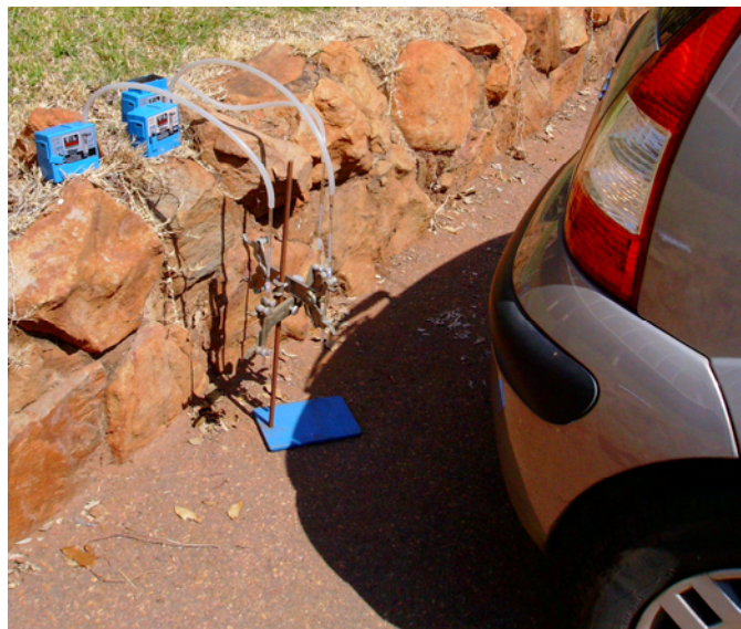
Figure 5.1: Sampling of diesel vehicle emissions with multi-channel silicone rubber traps and quartz fibre filters. Sampling configurations from left to right were: tube-filter-trap; trap-filter-trap and trap-trap.
