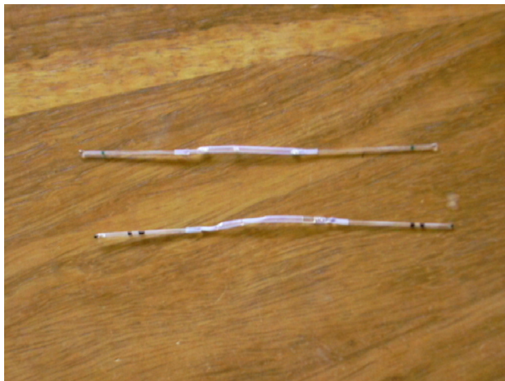
Figure 2.1: Examples of chlorobenzene permeation tubes.
