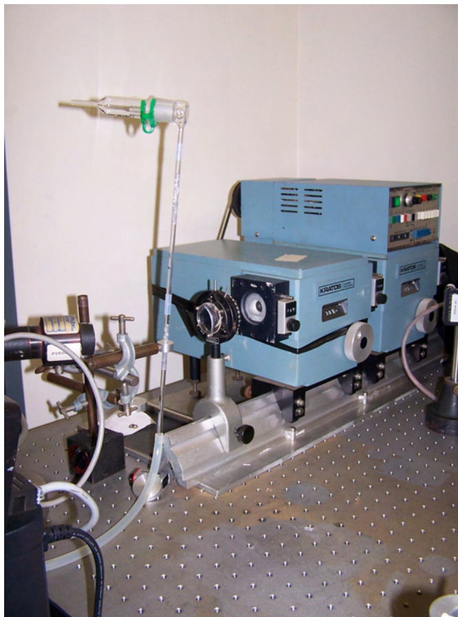
Figure 3.13: Experimental setup for the LIF breakthrough experiments. The naphthalene diffusion tube is mounted on two multi-channel silicone rubber traps in series, which are connected to a portable sampling pump. The monochromator is shown in the background.
