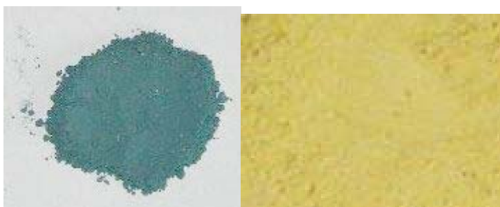
Figure 7-8: Fly Ash reacted with cobalt salt (left) and with 15 mass % \text{NH}_4\text{VO}_3 (right)
