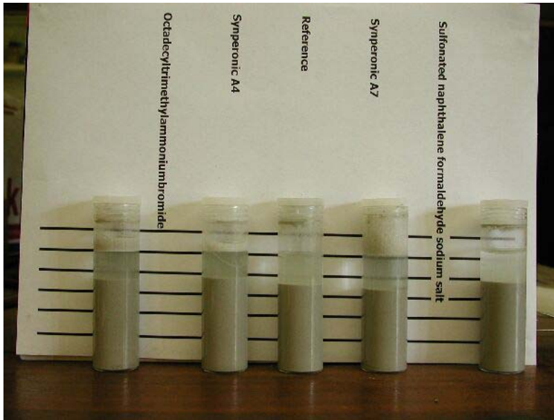
Figure 7-5: Octadecyltrimethylammonium bromide (successful), Synperonic A4 (successful), Synperonic A7, sulphonated naphthalene formaldehyde sodium salt used to suspend fly ash in water, after 5 minutes of settling time
