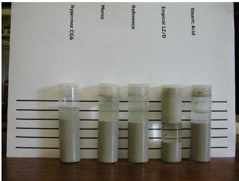
Figure 7-4: Hypermer CG6 (successful), Empicol LZ/D, Morez, and stearic acid used to suspend fly ash in water, after 5 minutes of settling time
