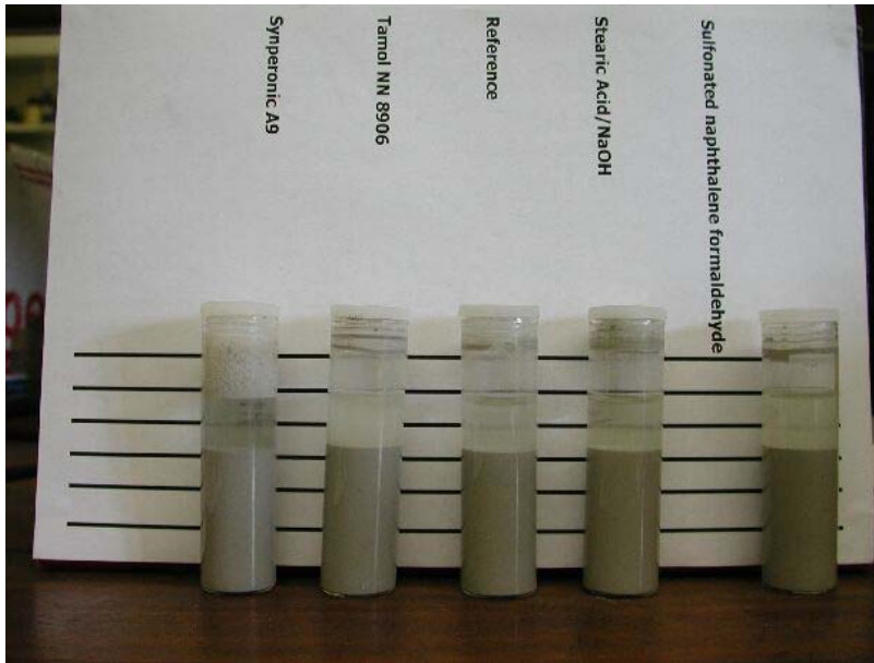
Figure 7-3: Synperonic A9, Tamol NN 8906, stearic acid/NaOH, and sulphonated naphthalene formaldehyde used to suspend fly ash in water, after 5 minutes of settling time
