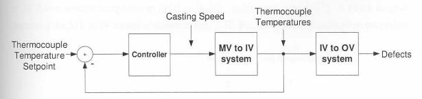
Figure 3.11 Block diagram description of the separation for control systems purposes.
