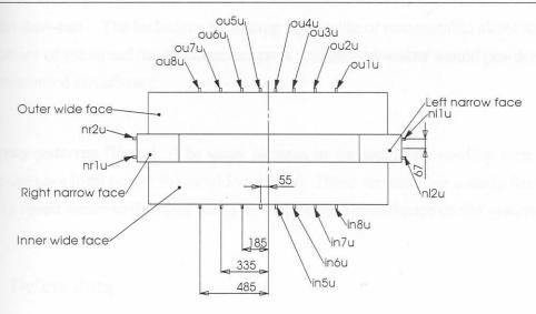
**Figure 3.2** Top view of the mould depicting location and naming conventions of the thermocouples. Note that in this view, the thermocouples shown are the top row of thermocouples. The bottom row of thermocouples have names "ou8*l*", "nr1*l*", *etc*.
