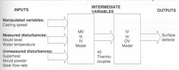
**Figure 3.10** Separation of system into two models, manipulated variable to intermediate variable and intermediate variable to output variable.
