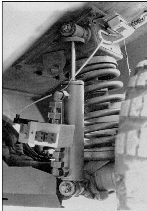
**Figure 1-4: Semi-active damper fitted to 4x4 test vehicle**
