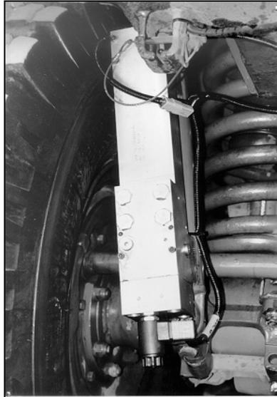
**Figure 1-6: Semi-active damper fitted to 6x6 APC**
