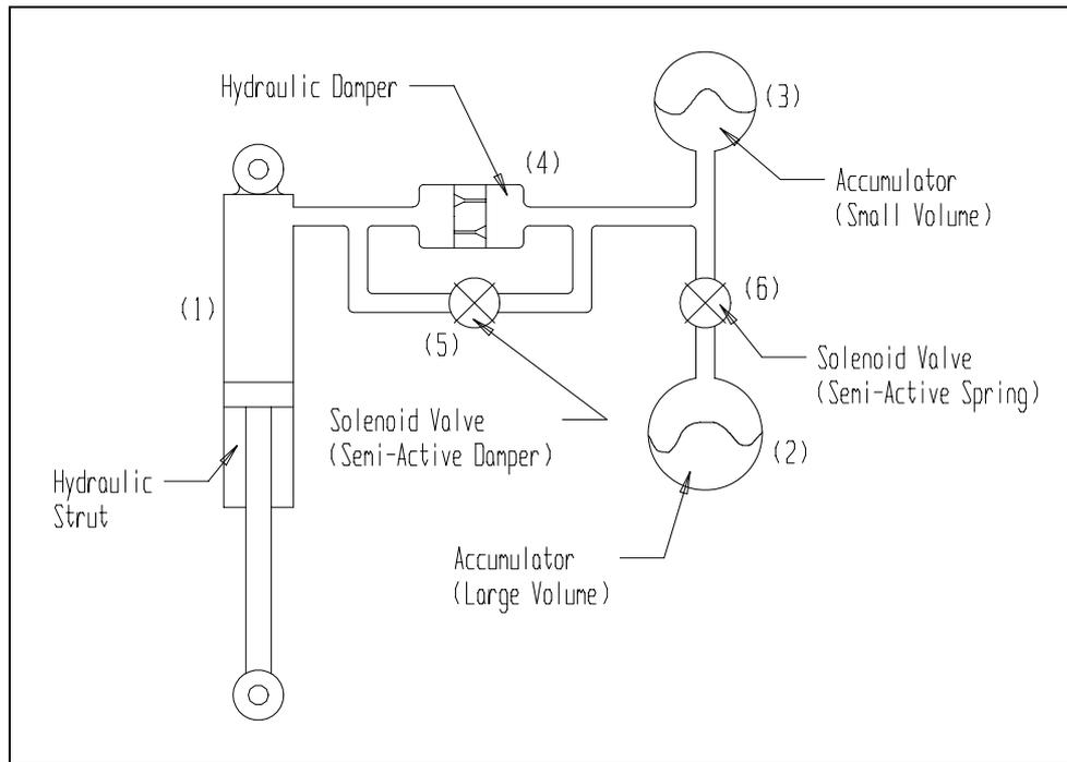
**Figure 1-10: Schematic layout of the semi-active spring/damper unit**
