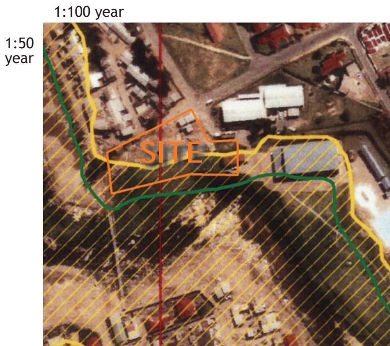
Figure 67 Until 2002, the 1:50y flood line was the official measurement for the building line. Since 2002, it has changed to the 1:100y flood line. As can be seen in the diagram, the 1:100y flood line covers many residential areas. (Source - ARP Infrastructure)
