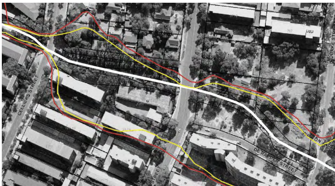
Illus. 28: The 50 and 100 year Walkerspruit floodlines between Bourke and Cilliers street. [Tshwane City Engineer, 2005]
