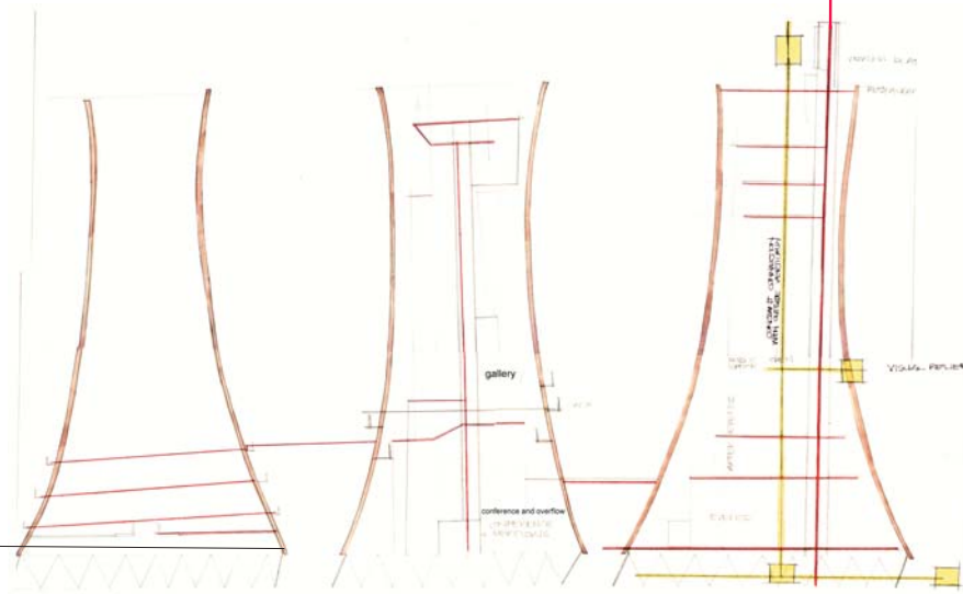
fig 6.7 Circulation routes within the towers
