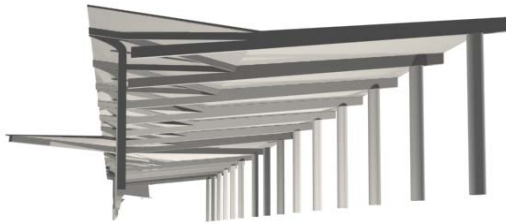
laminated wooden trusses
