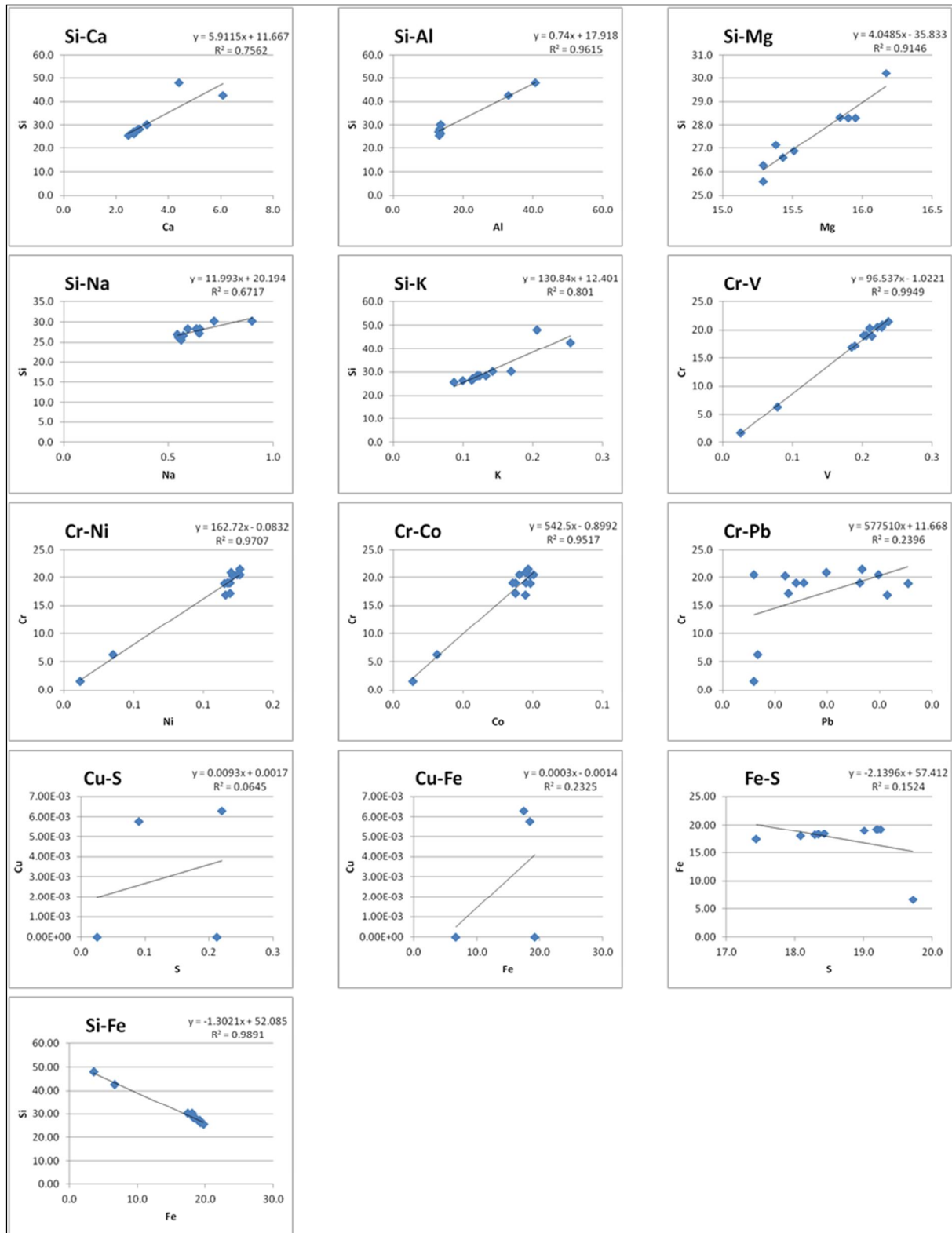
Figure 33: Correlation of major and trace element abundances obtained from XRF analysis.
