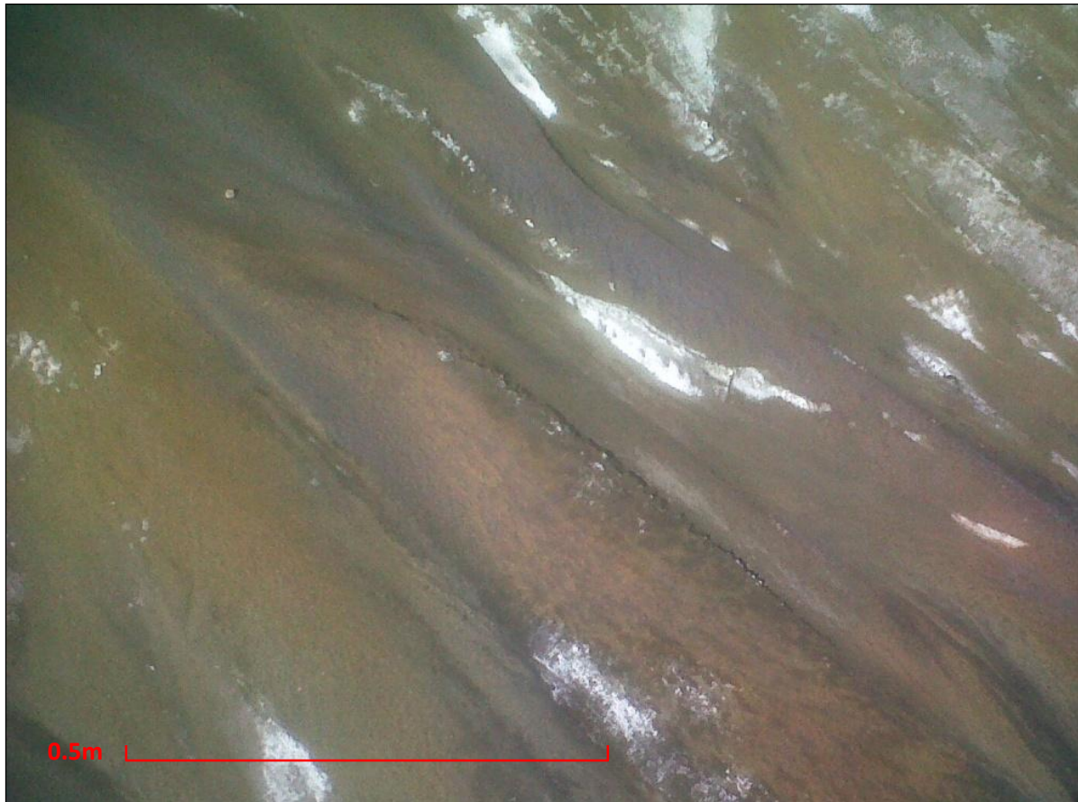
Figure 54: Precipitated salts and minerals on the tailings bank
