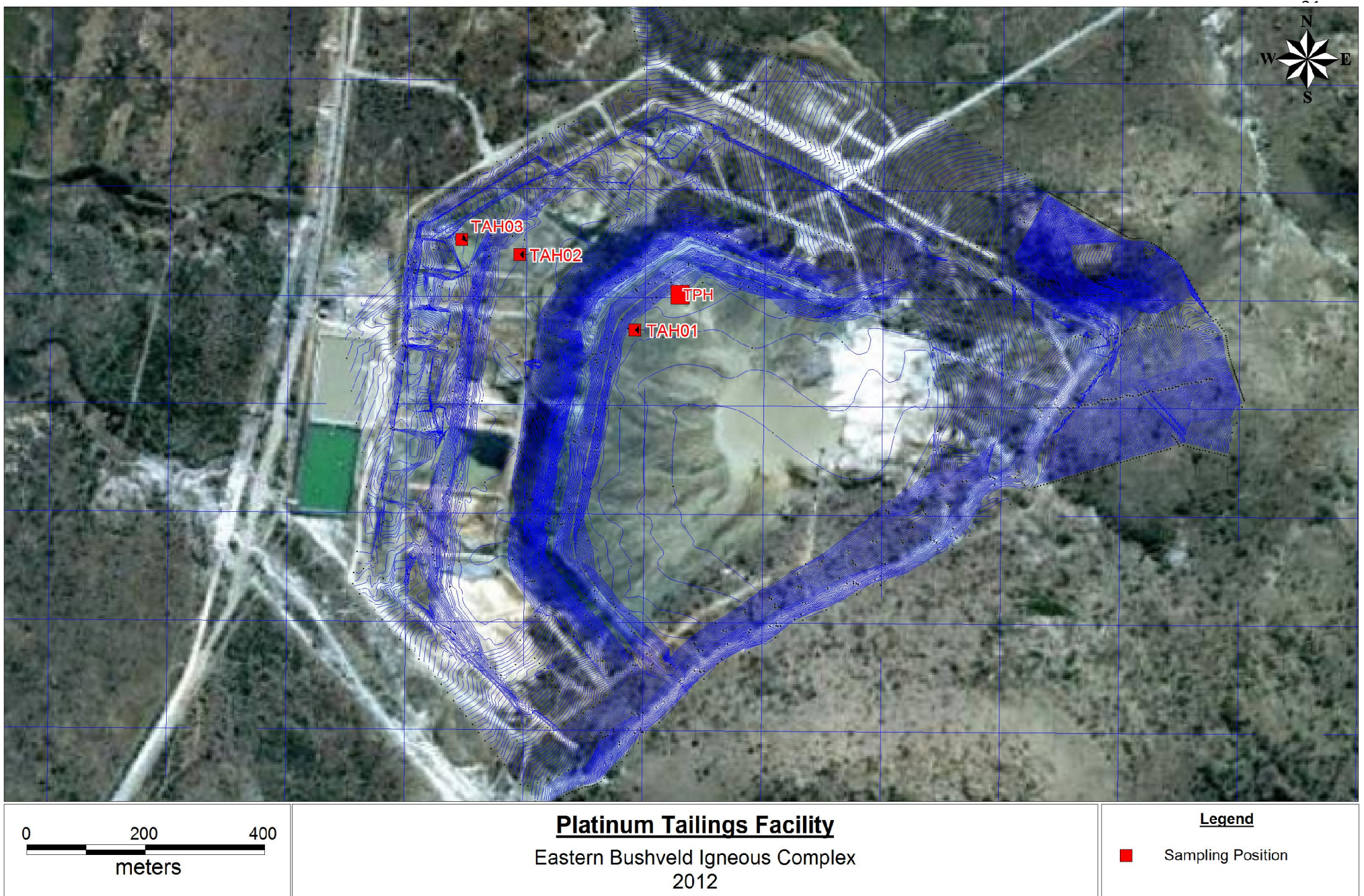
Figure 22: Aerial photograph of the tailings storage facility indicating sampling positions
