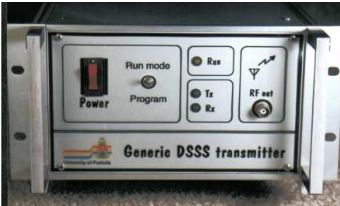
FIGURE 9.4: The complex DSSS transmitter unit (First hardware version).
