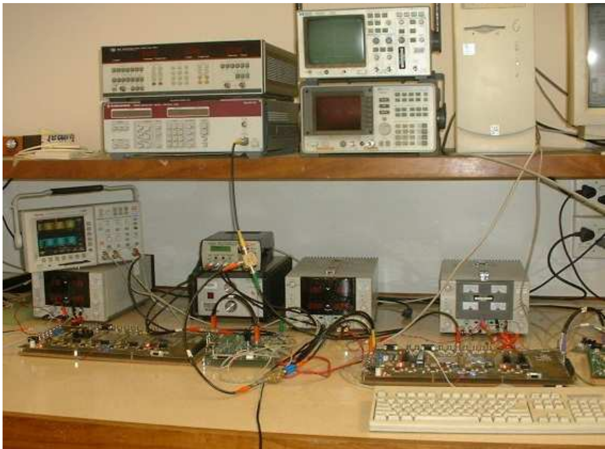
FIGURE 10.7: The hardware setup of the final DSSS modem employing CSS.
