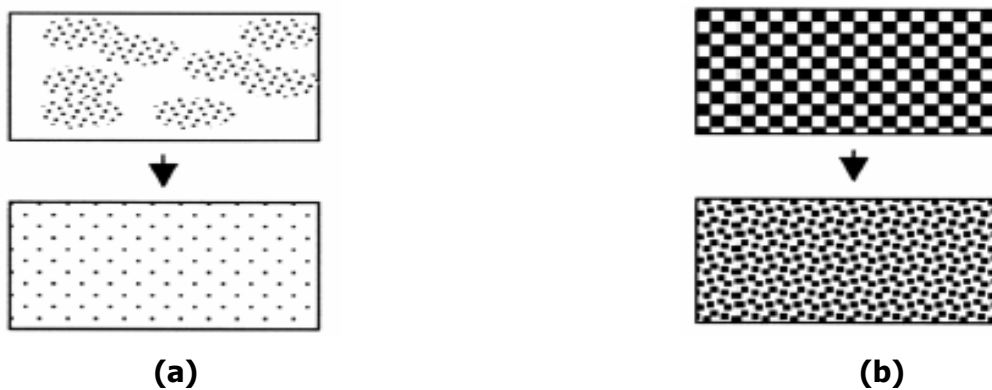
Figure 9: Two types of mixing mechanism: (a) distributive mixing, and (b) dispersive mixing (Chung et al , 2004).
