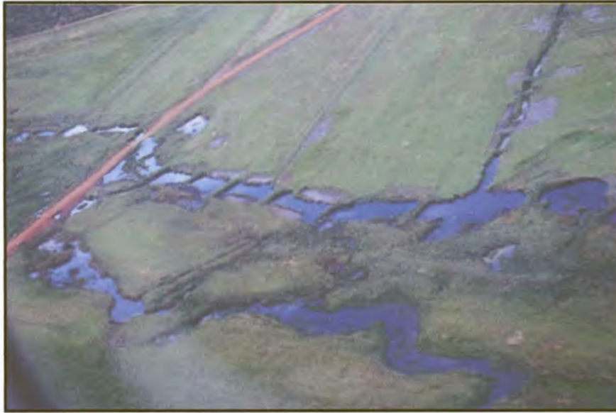
Figure 56: View of a flooded Zoar wetland. Note how the clay plugs act like dam walls (Photo: D. Lindley).
