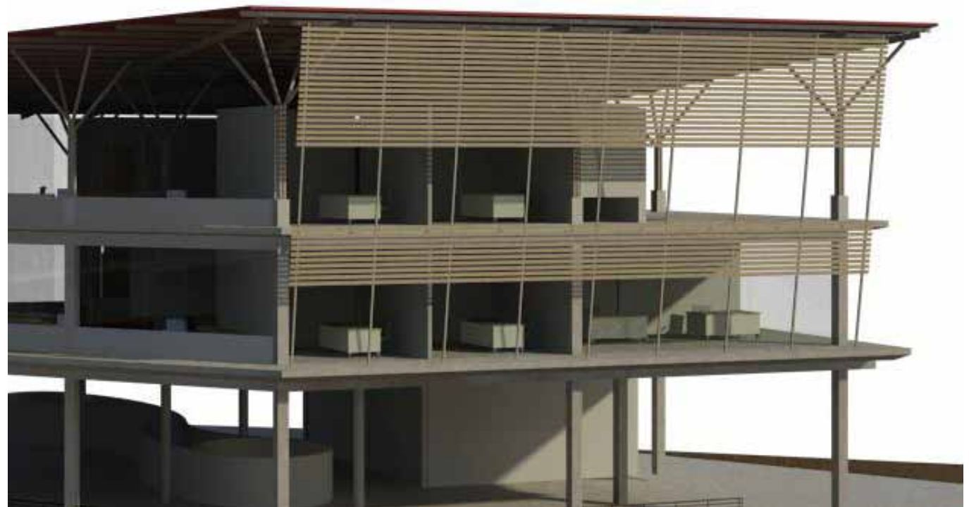
figure 152. 3d showing ecowood louvres on facade
