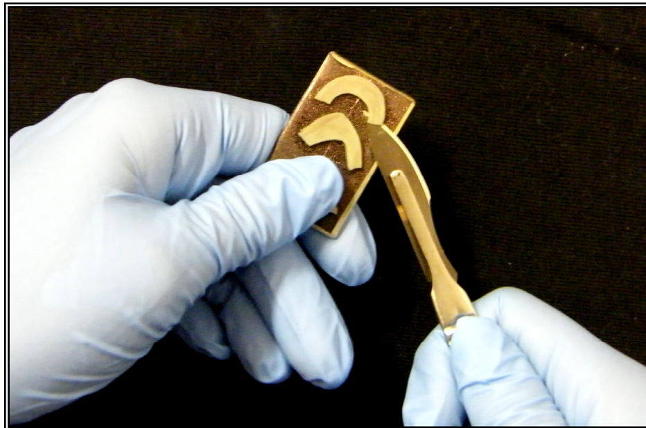
Figure 3.2 A scalpel bade was used to remove the bone samples from the metal slides.
