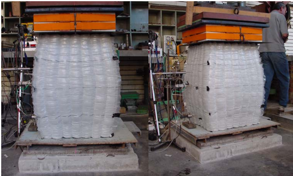
a) after 20% axial strain
