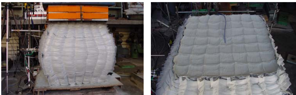
c) after 40% axial strain
