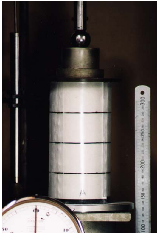
Figure 3.31 Single cell specimen in test machine.
