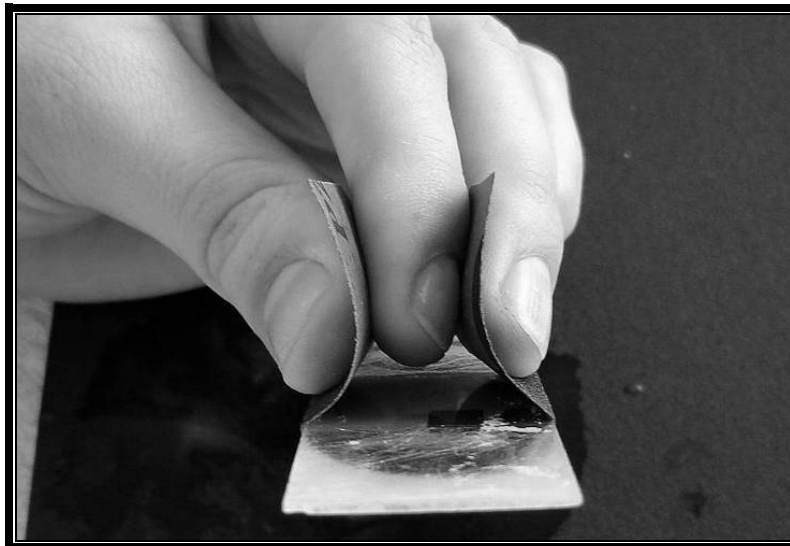
Figure 3.2 Illustration of Frost’s gripping device
