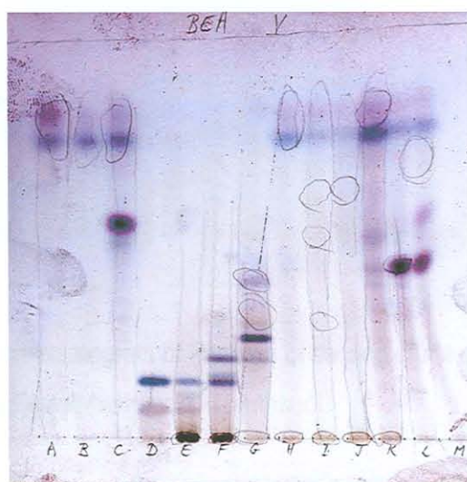
Figure 7.3. Thin layer chromatogram of the 13 combined fractions of Pteleopsis myrtifolia leaves, sprayed with 0.34% vanillin in 3.5% sulphuric acid in methanol.
