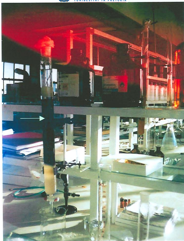
Figure 7.1. Photo of a silica gel column while eluting the chloroform fraction of Pteleopsis myrtifolia leaves with a mixture of hexane and chloroform (4:6).
