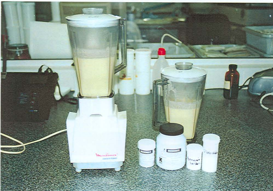
Plate 2 Curd slurry in liquidiser together with enzymes and other additives
