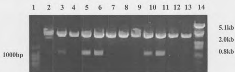
Figure 3.7 Restriction digestion analysis of p EucRTL2 recombinants. Lanes 1 and 14 contain the 100bp ladder (Promega) and \lambda HindIII/EcoRI marker, respectively. Lane 2 contains an undigested p EucRTL2 vector and lanes 3-13 represent putative recombinants p EucRTL2 -1 to p EucRTL2 -11 digested with NcoI and BamHI .
