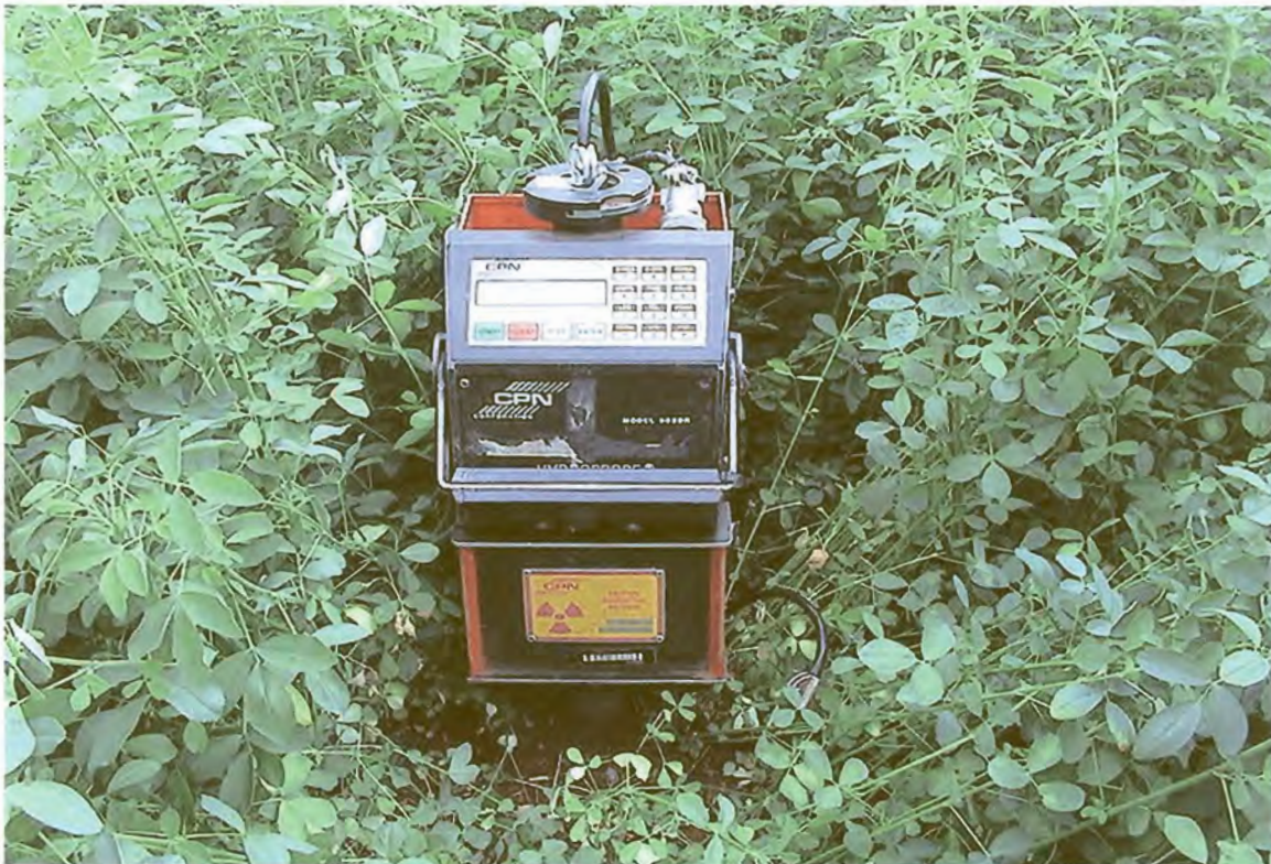
Figure 2.1 Neutron probe placed on the access tube. The probe is lowered down the access tube without exposing the operator to the radioactive source.
