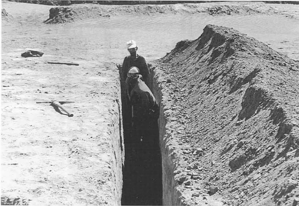
Figure 9: Photograph of the sampling trench in the tailings dam
