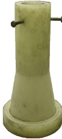
Figure 3.3. The 20° cone with changeable spigots. (Cone A)
