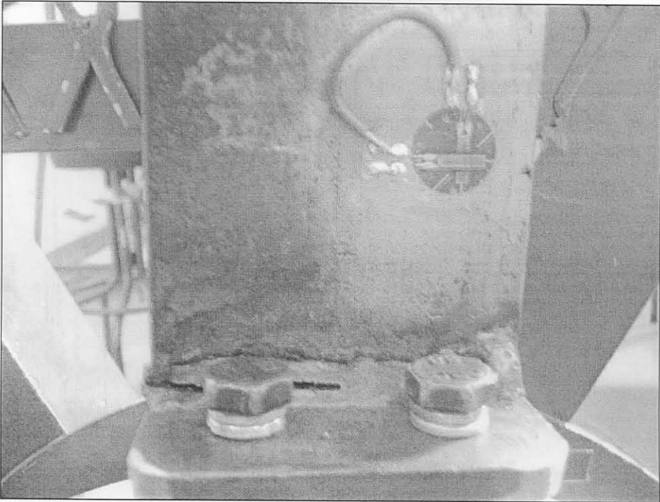
Figure D-3: Strain Gauge Rosette Orientation
