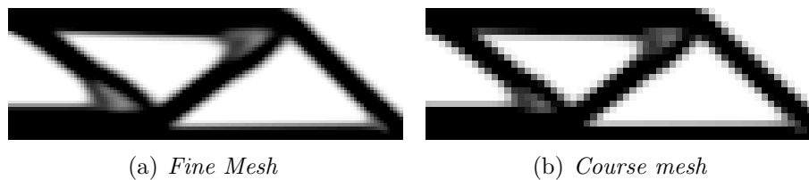
Figure 2.7: An optimized MBB-beam with different mesh discretizations. (The filter used in both sub figures has the same radius)
