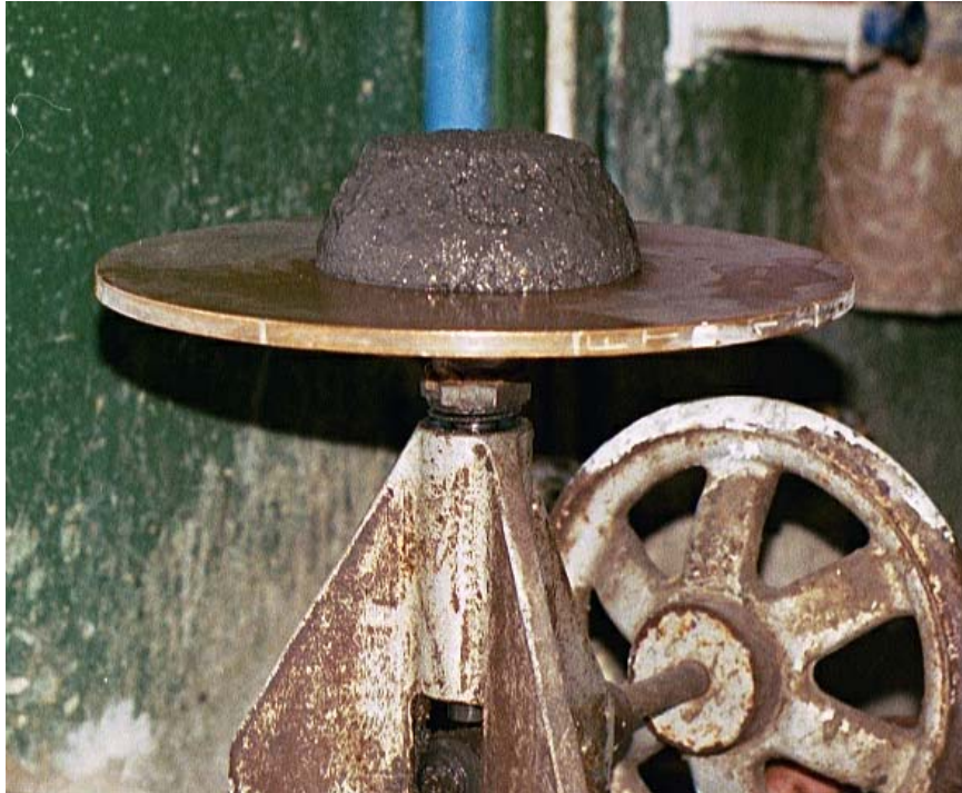
Figure 4.11 Photo of sample on flow table after mould is removed
