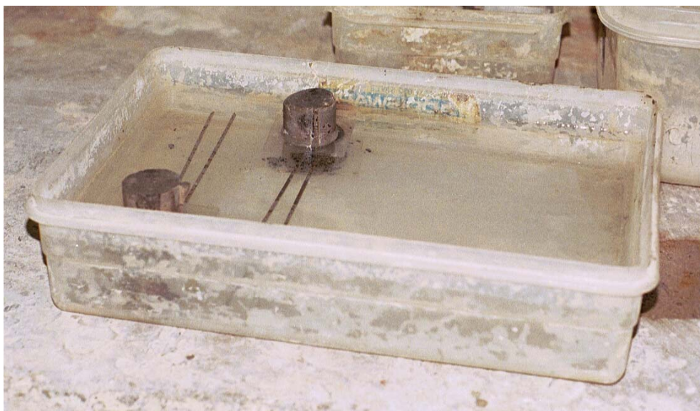
Figure 4.14 Le Chatelier moulds in humidity cabinet
