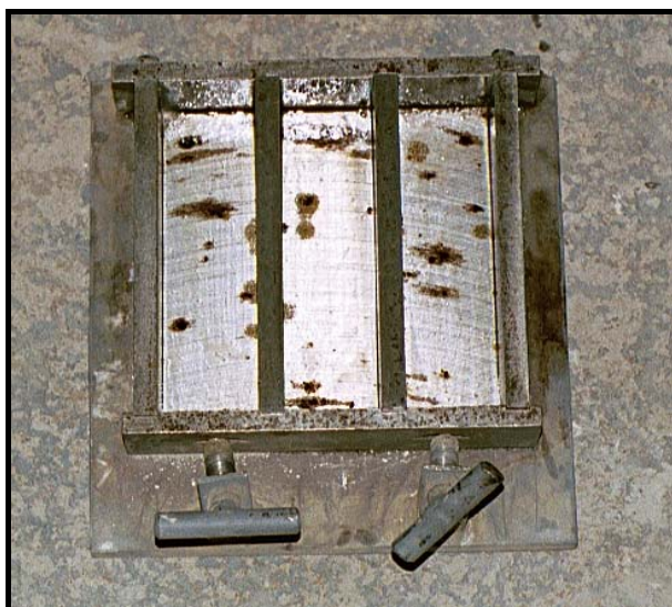
Figure 4.13 Photo of mould used
