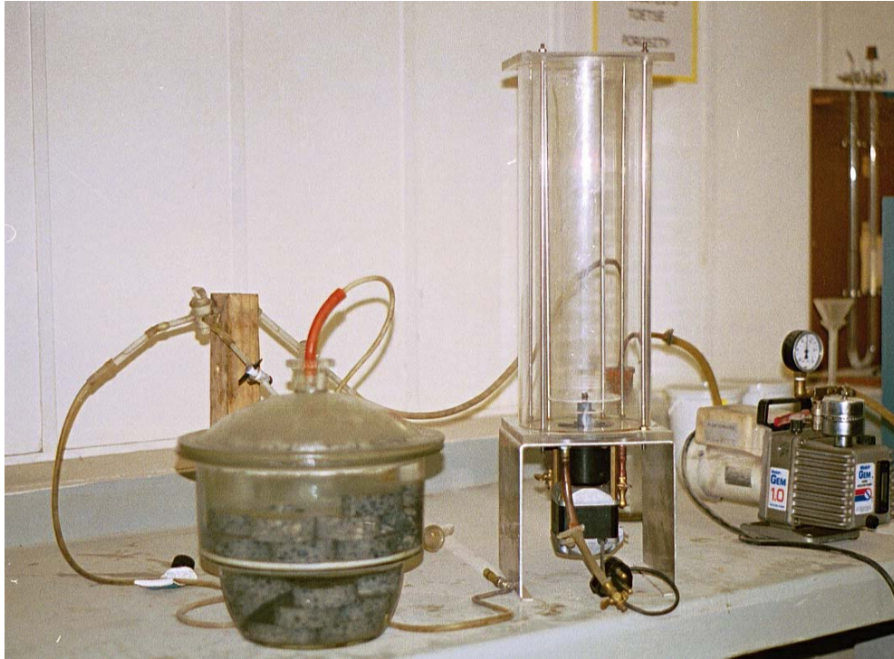
Figure 5.3 Photo of porosity test set up
