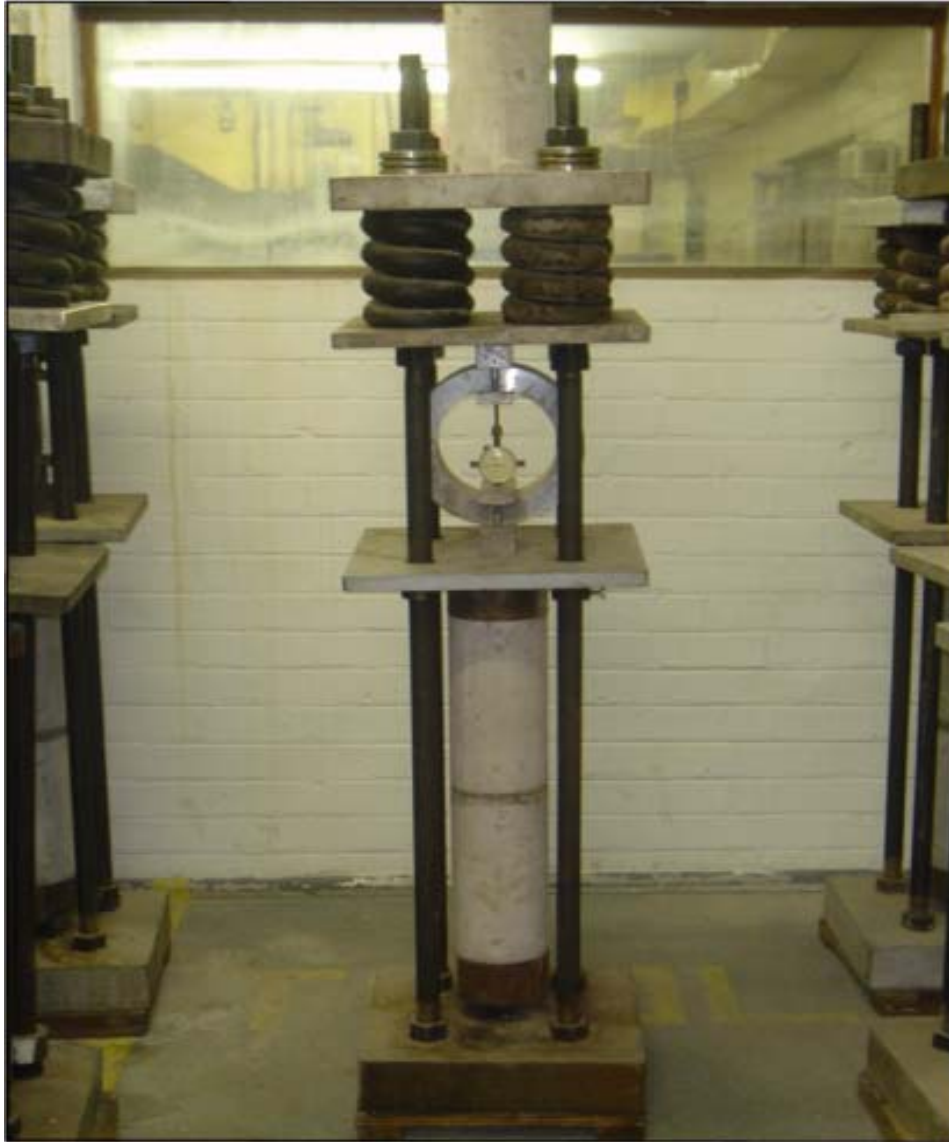
Figure 5.2 Photo of lab set-up for measuring shrinkage and creep
