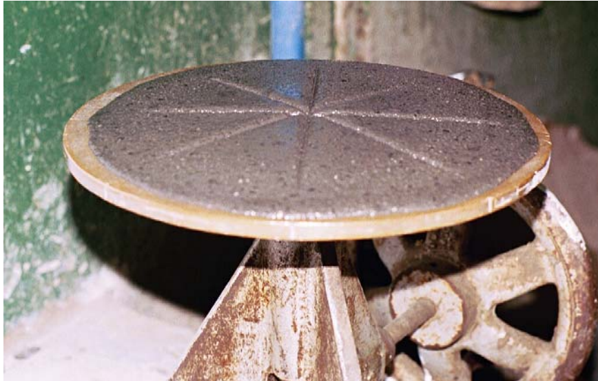
Figure 4.12 Photo of diameter measurements of flow table test
