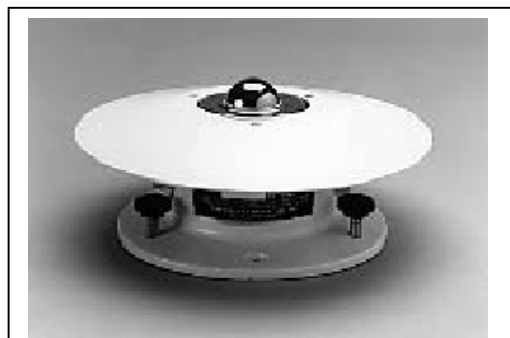
Figure 2.7 An Eppley Precision Infrared Radiometer
