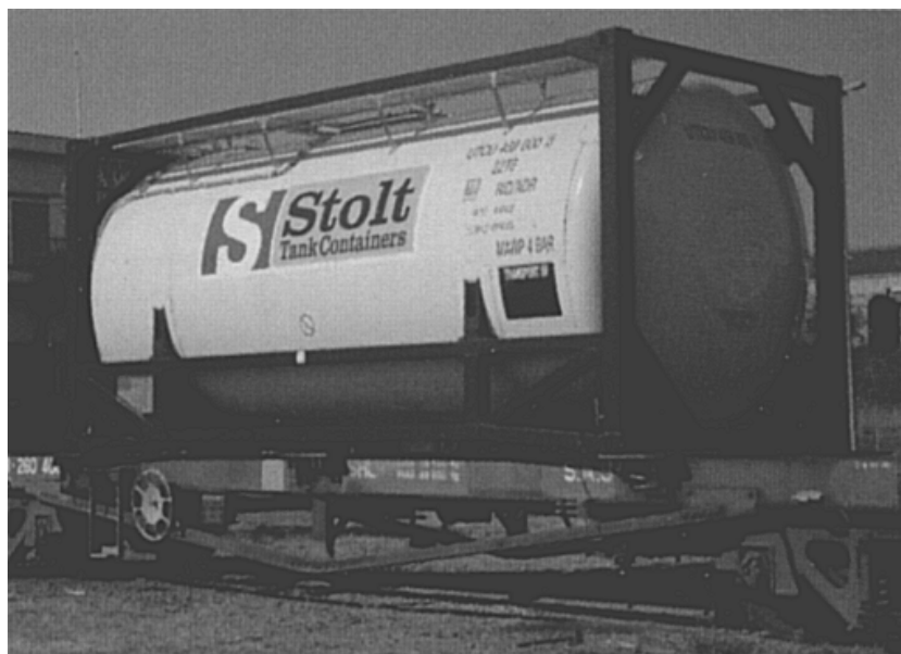
Figure 2-2 ISO tank container
