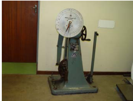
Figure 3.5. The Pendulum Impact Testing Machine
