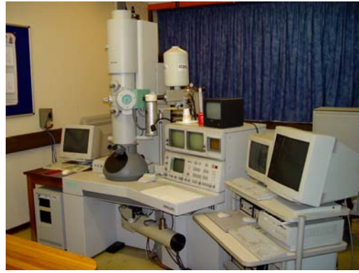
Figure 3.8. Transmission Electron Microscope PHILIPS CM 200
