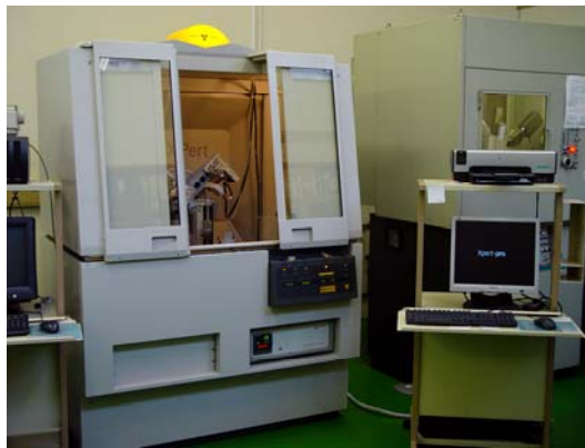
Figure 3.7. X-ray diffraction analyser X'Pert PRO PANalytical
