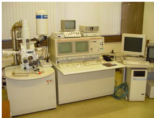
Figure 3.6. Scanning Electron Microscope JEOL JSM-6300, Model P90E.
