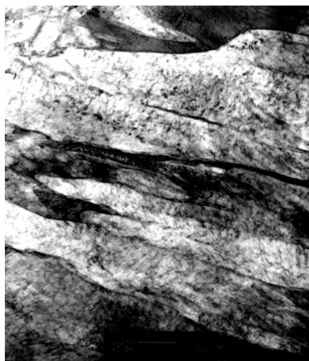
Figure 5.20: Thin foil TEM bright field image showing the precipitation of fine carbides in the matrix before the ballistic test of steel W tempered at 250°C for 15 minutes. Label mark 200 nm.
