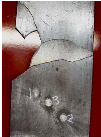
Figure 5.6: Untempered armour plate of steel U fractured by impact loading during ballistic testing showing the fracture some centimetres away from the impact points.
