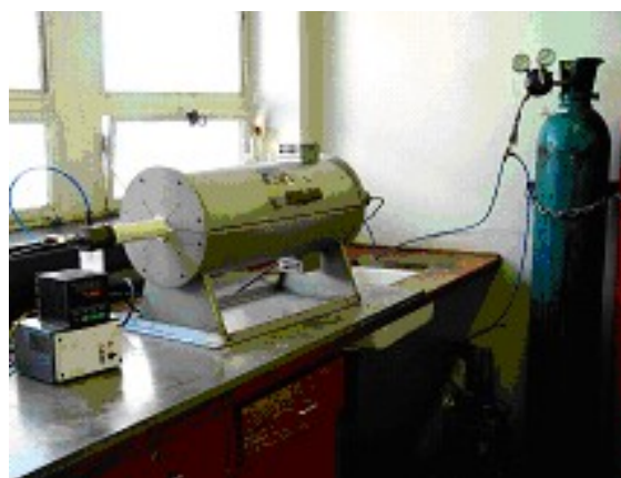
Figure 3.1. The tubular furnace LINDBERG MK-1018 for austenitisation
