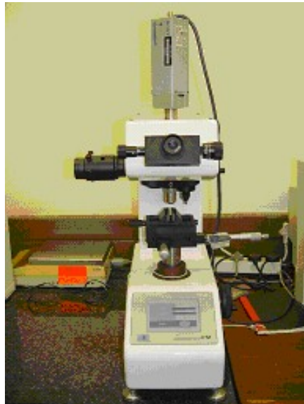
Figure 3.2. Microhardness Tester FM F11-1
