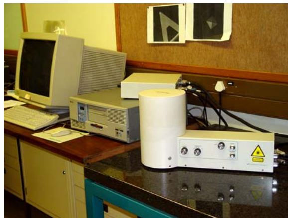
Figure 3.9. Atomic Force Microscope: Topometrix TMX 2000 “Discoverer”
