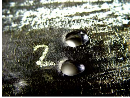
4.4.34(c):. Front of Steel F plate after firing
