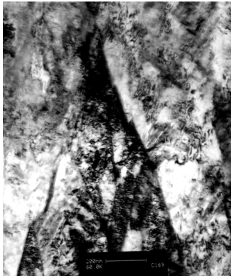
Figure 4.4.40: Bright field thin foil transmission electron microscopy of steel H tempered at 300°C showing the cementite
