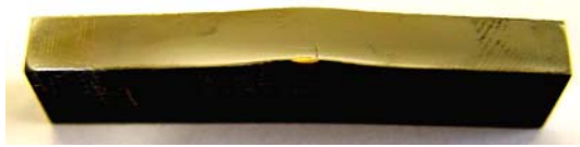
Figure 5.4: Cross section throughout the affected impact region showing the copper from the round attached on to the front face of a 4.8 mm steel W plate. The bending of the plate in the affected impact region is also observable.
