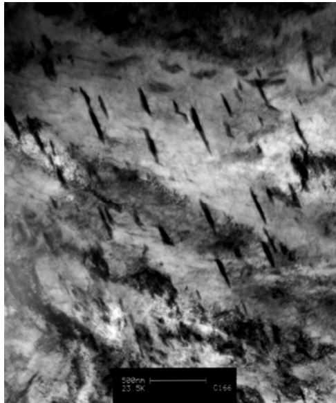
Figure 4.4.41: Bright field thin foil transmission electron microscopy of steel E tempered at 400°C showing large strings of the cementite.
