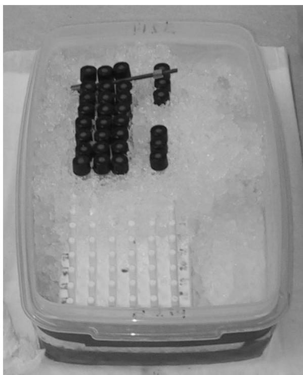
Figure 15. Reaction vial racks. Shown with pegs sawn off for easier handling of the reaction vials.
