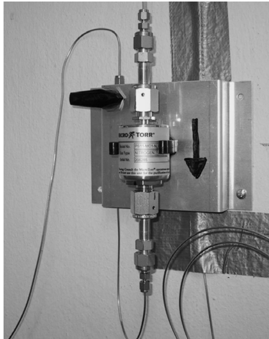
Figure 8. SAES Getter. Used to filter gas for purging reaction vials prior to instillation of tissue homogenate to ensure a zero CO baseline.
