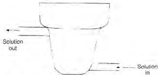
Figure 3.1: Flow cell with a volume of 30 ml to fit on a PARC Model 303 SMDE
