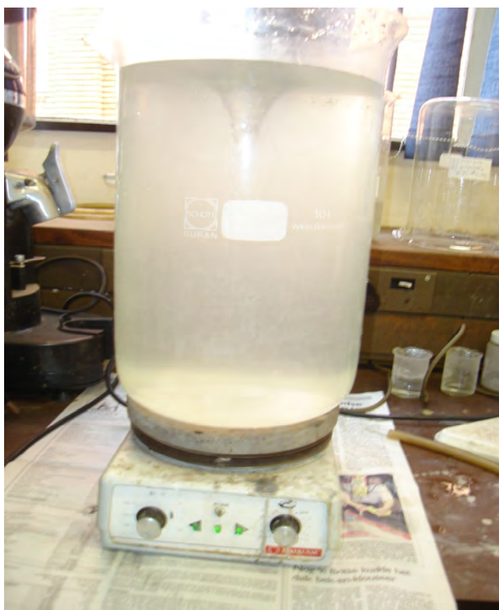
Figure 42: A month-old dispersion of cypermethrin pellets in 10 L of tap water showing stability (absence of phase separation)
