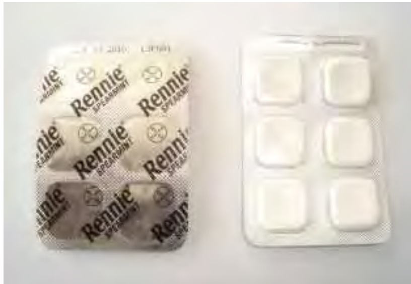
Figure 4: Illustration of both sides of the same blister pack. The transparent thermoformed plastic sheet containing cavities for each unit dose (placed on the right) is the base material. An aluminium covering foil is laminated and sealed with the rigid plastic sheet, as showed on the left.
