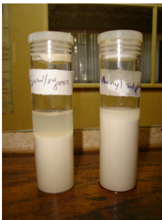
Figure 31: Cypermethrin dispersion with Emulsogen EL only (on the left); and cypermethrin dispersion with a blend of Emulsogen EL and Phenyl Sulphonate CA (on the right). A better emulsion was obtained by blending the surfactants.
