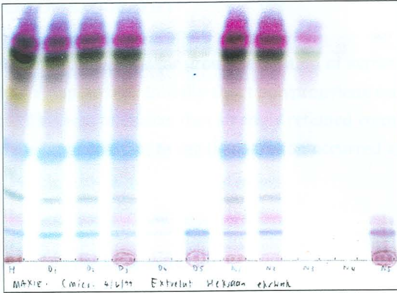
Figure 3.13 Separation of components in 50 \mu\text{g} of the different Extrelut fractions using the BEA eluent and the vanillin spray reagent. From left to right: H = hexane fraction, D1-D4 = dry adsorbent fractions eluted with hexane, D5 = dry adsorbent fraction eluted with acetone, N1-N5 = wet adsorbent fractions eluted with hexane and N5 = wet adsorbent fraction eluted with acetone.
